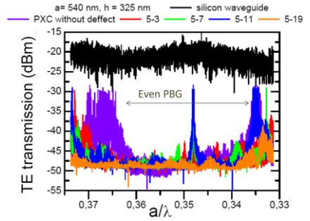
**Figure 2:** Measured spectra of a fabricated sample. The calculated PBG for even modes is shown. The peaks appearing in the PBG correspond to modes localized in the cavities.
