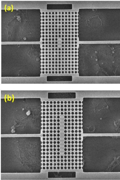
**Figure 1:** SEM images of a suspended square lattice silicon photonic crystals with cavities created by removing N holes in the transversal direction. (a) N=3 and (b) N=11.
